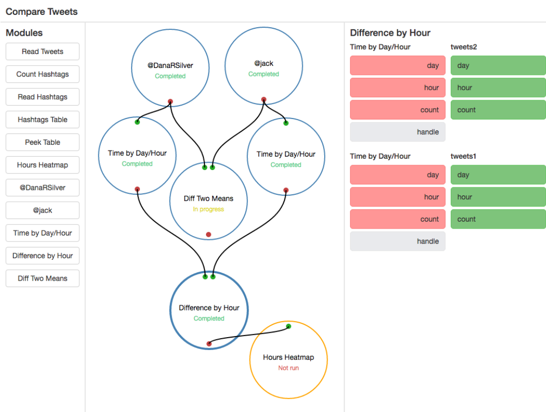
Figure 4.3: MiddGuard’s graph editor user interface, open on a graph named “Compare Tweets”. On the left, the modules panel lists all loaded modules, from which nodes can be created. In the center, the graph editor canvas has seven nodes initialized from their respective modules, and connections between the nodes. On the right, the detail panel shows the column mappings between the “Difference by Hour” node and its connections to two “Time by Day/Hour” nodes.
